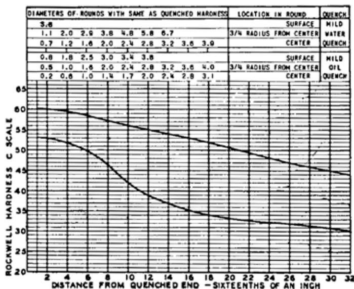
Figure 3: Diameters of Rounds with the same as-quenched hardness, as a function of the distance from the quenched end for ASTM A304 [3].
