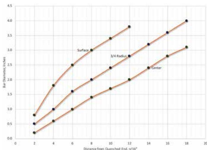
Figure 2: Typical Jominy End Quench Data of SAE 4140H plotted in accordance with ASTM A304 [3].
