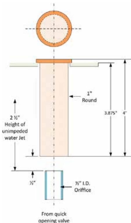
Figure 1: Schematic of the Jominy End-Quench Apparatus.
