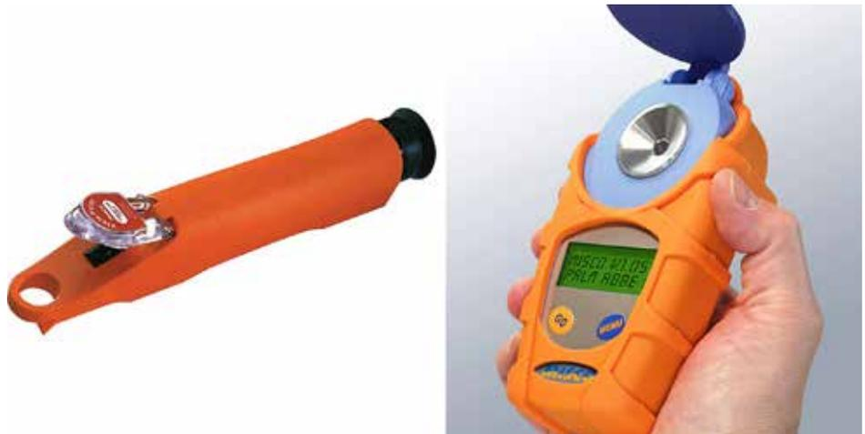
Figure 1: Typical analog and digital refractometers.
