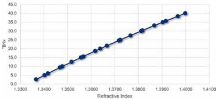
Figure 2: Relationship between refractive index and °Brix.
