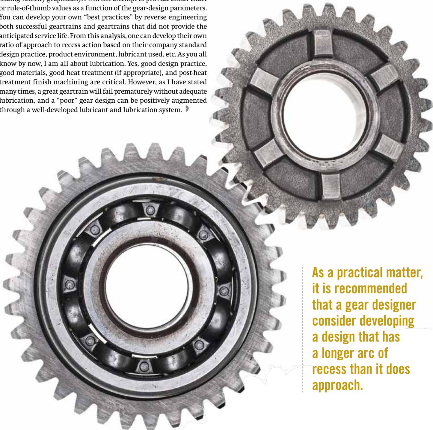
**As a practical matter, it is recommended that a gear designer consider developing a design that has a longer arc of recess than it does approach.**
