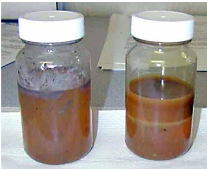
Figure 2: Typical contaminated polymer quenchant.
