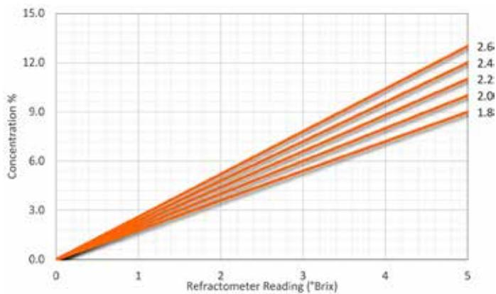
Figure 3: Typical refractometer versus % concentration based on different multiplying factors.
