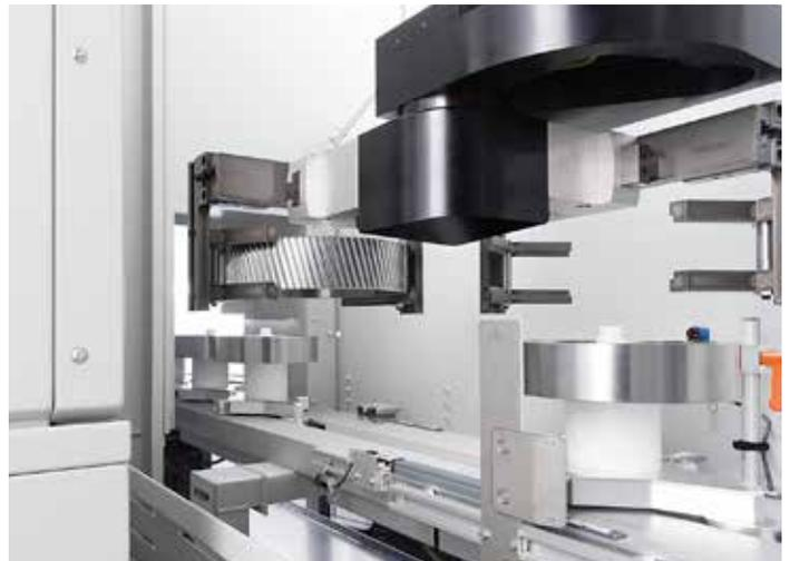
While the 280H is available with a 2-station ringloader, the 280HCD features an additional gantry loader to link gear hobbing with chamfer cutting and external automation/storage. (Courtesy: Gleason)
