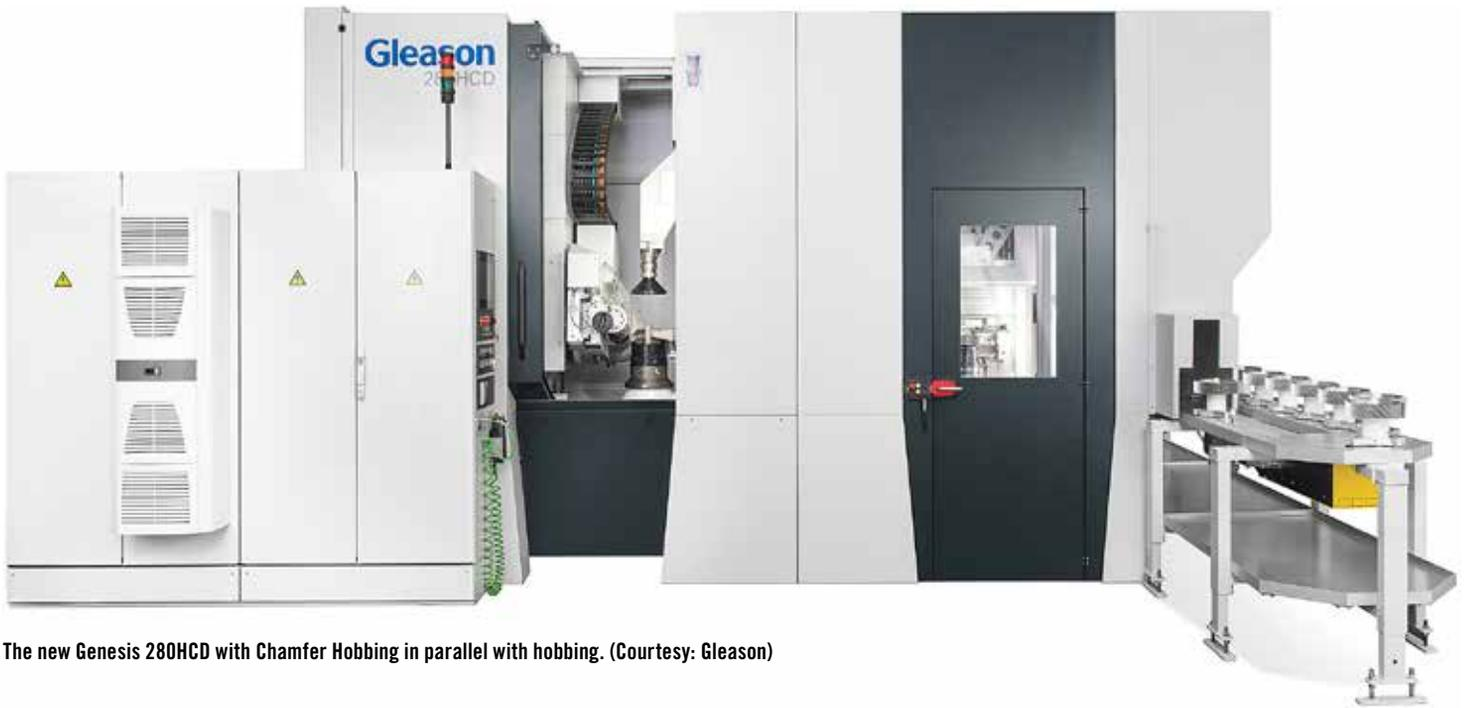
The new Genesis 280HCD with Chamfer Hobbing in parallel with hobbing. (Courtesy: Gleason)
